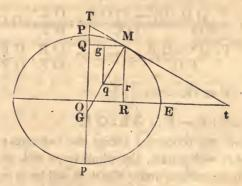
For if P E p P be a fluid, P p the axis round which it revolves, then may the spheroid revolve in such a time that the centrifugal force of any particle M combined with its gravity, may make this whole force act perpendicularly to the surface. For let E = attraction at the equator, P = attraction at the pole, F = centrifugal force at the equator.
